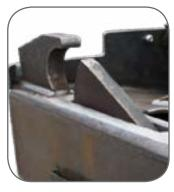
Automatic spring loaded front container lock helps ensure containers remain in place.
