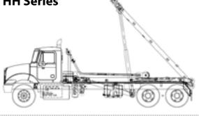
HH - A shortened and narrowed version of the OR-model that is designed to pick up deadlift containers with a knuckle cable end. The hoist rails are set at 35 inches wide.
