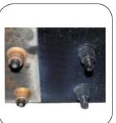
Hoist frames are huck bolted to chassis, providing unmatched strength and durability (factory mount only).
