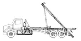
A representative of a unique market sector of the TM-model (Trough Mount) is typically a hoist that utilizes a trough section on either side to support the containers as opposed to rollers or rails. Many different variations exist for its dimensions and can be adapted to suit most consumer requirements.
