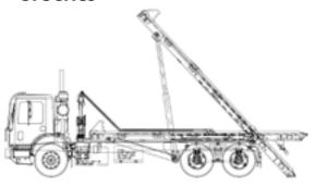
A cross breed of sorts, the SI-model is unique in the fact that it is designed to pick up a variety of different styles of containers. Specifically it will pick up either outside rail, inside/outside rail and deadlift containers. The hoist is set at 34 inches.
