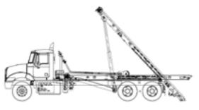
Similar to the OR-model, the IO-model has additional inside rollers (inside of main frame tubes) and inside rails fixed to the top of main frame. The hoist is set at 35.5 inches wide between rails.
