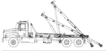
A combination of an EX & HH-model, designed for picking up dead lift containers at low loading angles with an 80" extendable tail section. This hoist has a narrower rail width set at 35 inches.
