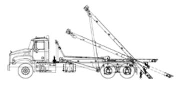
An OR-style hoist with a tail that is extendable out to an additional 48". The hoist has set rail widths of 35.5 inches.
