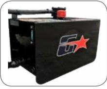
Oil reservoir equipped with 10 micron breather filter; 3 micron oil return filtration; 100 micron mesh screen suction strainer and fluid level indicator with temperature gauge.
