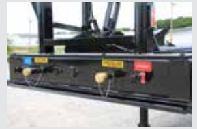
7-Wire Electric Trailer Plug Connection; 5-Wire Electric Pig Tail Connection; Turn Lock Quick Disconnect Air Lines; 1 1/4" Return Line w/ Quick Disconnect Threaded Male End; 1" Pressure Line w/ Quick Disconnect Threaded Female End
