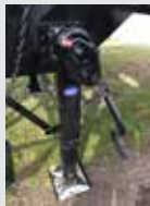
50k lb. Lift / 140k lb. vertical load twin leg manual landing gear
