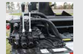
Manual controls mounted to front fender on driver's side
