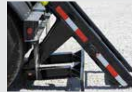
Auto folding mechanical ICC bumper with rear impact energy absorption
