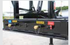
7-Wire Electric Trailer Plug Connection; 5-Wire Electric Pig Tail Connection; Turn Lock Quick Disconnect Air Lines; 1 1/4" Return Line w/ Quick Disconnect Threaded Male End; 1" Pressure Line w/ Quick Disconnect Threaded Female End
