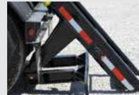
Auto folding mechanical ICC bumper with rear impact energy absorbtion
