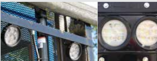
Additional LED Work Lighting (front and rear)
