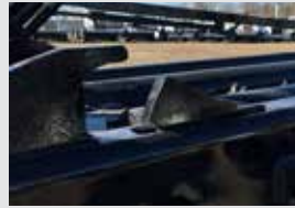
Automatic Spring Loaded Pass Over Front Container Safety Lock
