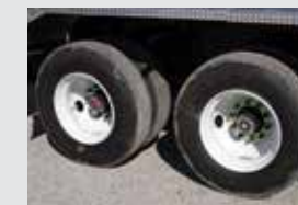
10-Hole Hub Piloted Steel Rims w/ 11R/22.5 Tires - 16 Ply & Wheel Check Indicators
