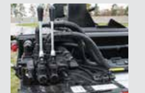
Manual controls mounted to front fender on driver's side
