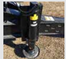
Hydraulic single leg landing gear
