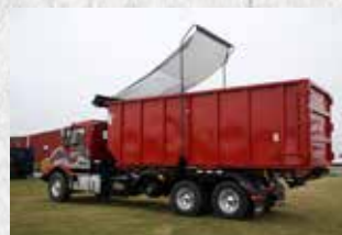
U5-OR-174 shown with Pioneer® tarp, front and rear ratchet hold downs, lift axle, and poly tri-axle fender options
