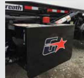
Steel hydraulic tank side mounted with 3 micron filtration, dual sight/temp. gauge & air breather
