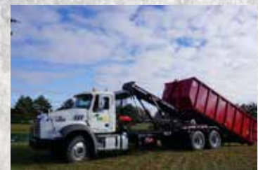
U5-OR-174 shown with Pioneer® tarp, LED safety lighting, Hi-Vis yellow tail, rear ratchet hold downs, rear window screen, fire extinguisher, and poly tandem axle fender options
