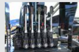
Inside air controls in power tower or integrated into center console on cab over trucks; Secondary outside manual controls at main control valve
