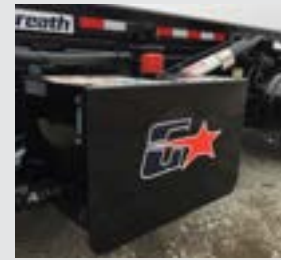
50-gallon steel hydraulic tank side mounted w/ dual sight/temp gauge
