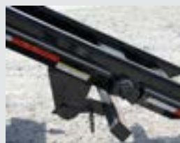
Air assist auto folding ICC bumper
