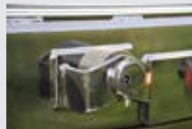
Outboard supported side rollers (standard on 75k lb. and up models)
