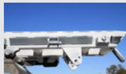
Rear wing skid plates w/ Heavy-duty nylon ratchet rear container hold downs
