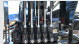
Inside air controls in power tower or integrated into center counsel on cab over trucks w/ in cab hoist up light; Secondary outside manual controls at main control valve
