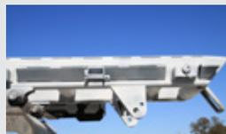
Rear wing skid plates w/ Heavy-duty nylon ratchet rear container hold downs
