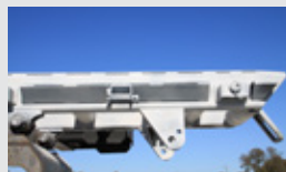
Pintle adaptable heavy-duty rear apron w/ split bumpers & recessed LED lights
