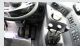
Inside air controls in power tower or integrated into center console on cab over trucks w/ in cab hoist up light; Secondary outside manual controls at main control valve
