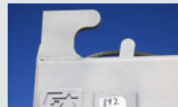
Automatic pass over front container safety lock & 1 1/4" steel front stops
