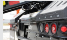
Pintle adaptable heavy-duty rear apron w/ split bumpers & recessed LED lights
