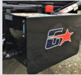
Steel hydraulic tank w/ in tank 3 micron filtration and a dual sight and temperature gauge; competitor's filter on left & Galbreath's on the right
