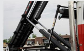
Reverse mount, inboard above frame lift cylinders
