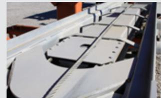
Fully protected single cylinder winch rail design
