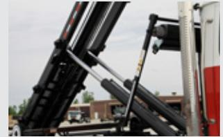
Reverse mount, inboard above frame lift cylinders
