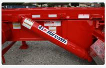
2 cylinders are mounted on the outside of the rails to provide stability when loading/unloading heavy boxes.
