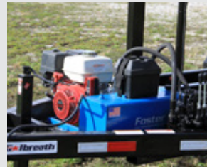
8,000 lb. top wind jack; 12HP Honda engine w/ electric start; 9-gallon hydraulic tank; 25 gpm manual control valve
