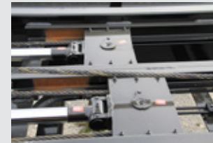
Dual reaving system with UHMW guides
