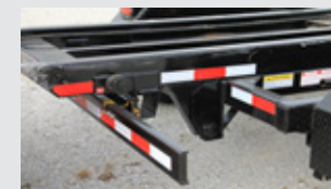
Rear impact protection bumper as required by DOT regulation
