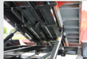
Dual lift cylinders for hoist frame
