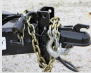
Adjustable hitch with safety chains, 7 pin trailer connector and emergency breakaway
