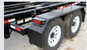
Tandem single tire 7,200 lb. axles covered with steel tandem fenders and recessed LED lighting
