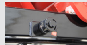
3" OD outside rail rollers w/ bronze grease grooved bushings
