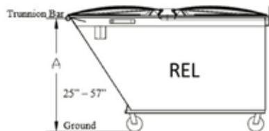
The SLCH models have been optimized for use with 25" pocket heights on FEL type ANSI compliant containers. The SLCH-X models were developed to be compatible with FEL containers that have fork pocket openings ranging from 17" up to 44.5" and REL containers with trunnion bar heights ranging from 45" up to 49".
