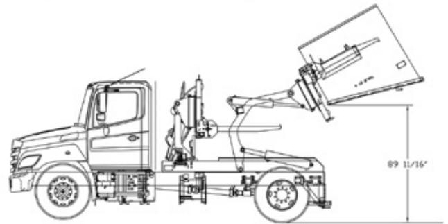
\* Only FELs can be rotated. Minimum chassis requirement 25,000 (10,000 front and 15,000 rear). Based on ANSI compliant containers of standard construction within manufacturer's maximum load and weight rating. Based on truck with 4,910 lbs. front and 183" WB with static water level loads.
