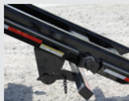
Air assist auto folding ICC bumper
