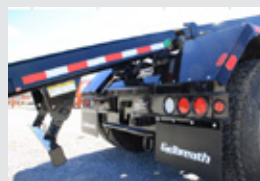
Heavy duty rear apron w/ split bumpers & recessed LED lighting
