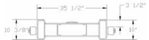
HOIST FRAME DETAIL
