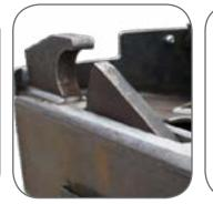
Automatic spring loaded front container lock helps ensure containers remain in place.
