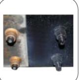
Hoist frames are huck bolted to chassis, providing unmatched strength and durability (factory mount only).
