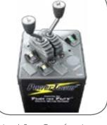
In-cab Power Tower featuring "plug n' play" wiring and smooth hydraulic activation through air over hydraulic controls.
