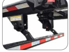
Air assist ICC bumper standard on most cable hoists models (no applicable on HH, EX, EH, IX models; available auto folding ICC bumper as option only; see Available Options below).
